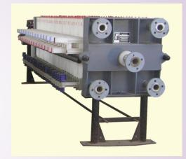
In the recessed type, the slurry is fed through the central inlet and the solids are retained in the recess between the plates, while the filtrate is collected through the corners.
